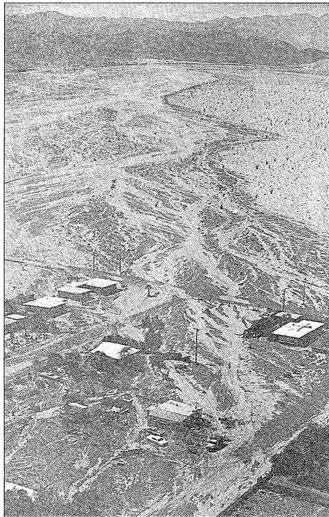
Figure 2. Damaged homes on a fan in Ocotillo Wells, California, which lies in eastern San Diego County. Tropical Storm Kathleen caused extensive flooding September 9-11, 1976, there and throughout Riverside and Imperial counties to the north and east. The channel braiding shown in the photo is typical of alluvial fan flooding, and thus it is difficult to predict the location of floodflows.
